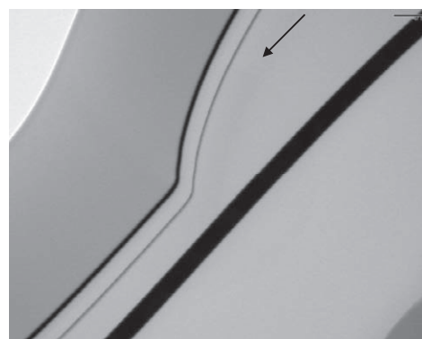
Fig.3 Cross sectional TEM image of OLED display Sample is prepared by FIB fabrication.
